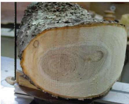
Figure 4. Using a Delta circle-cutting attachment to cut out the bowl blank.
