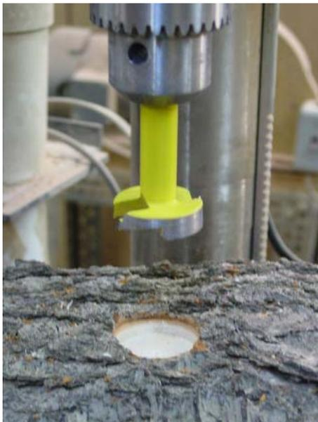
**Figure 5. Drilling a small hole for the spur drive center.**
