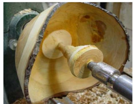
**Figure 17. Cutting away the spigot in the center.**
