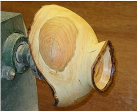
**Figure 12. At this point, a bit more rough sanding is needed.**
