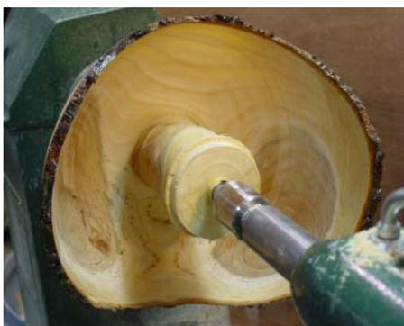
**Figure 7. Rough hollowing the center leaving a spigot for the chuck to grip when turning the bottom of the bowl.**
