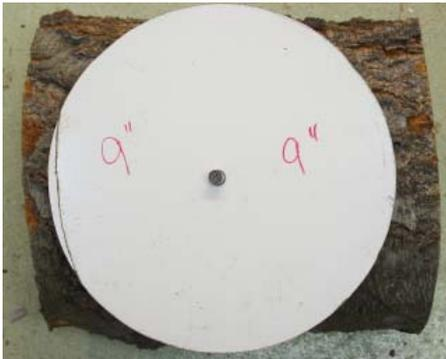
Figure 3. Log section with masonite disk to mark the piece to be cut on the bandsaw.
