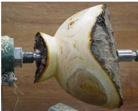
**Figure 6. Mounted between centers and the outside turned.**
