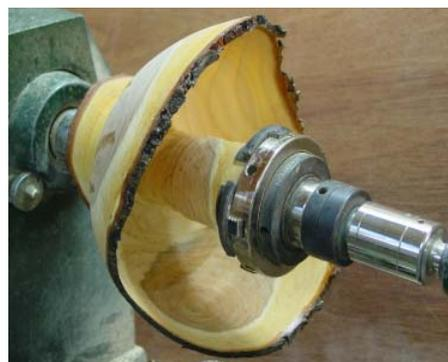
**Figure 8. Chuck gripping the spigot while still on the spur drive.**
