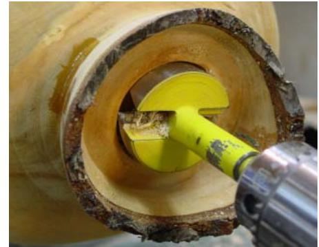
**Figure 9. Drilling a recess in the base to provide a place to grip the bowl while the spigot is removed from the inside.**
